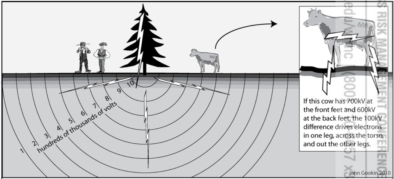
Fig. 3: **Ground current** causes roughly half of all lightning injuries to humans. The difference in voltage between one foot and the other drives current through us. In this simplified illustration the cow has a 100kV (100,000 volts) differential, one farmer has a 50kV differential, and the other farmer has her feet together so her voltage difference is close to zero. See Uman's book (2008, ch.5) for a more precise representation of ground current distribution.
