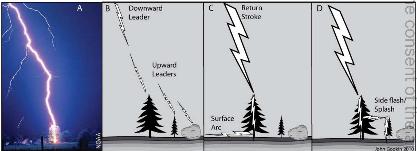
Fig. 4: A) A typical lightning strike to a tall tree. There are two upward leaders that did not attach to the downward leader. B) Some **upward leaders** do not attach to the downward leader but still carry hundreds of amps and are quite dangerous. C) A **surface arc** is associated with ground current and can go tens of meters from the strike point. D) **Side flash** splashes some of the current onto a nearby object as an additional path to the ground.
